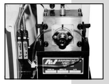
As the O-Ring passes through the O.D. Lubricator, the edges of the foam contact the O-Ring and deposit additional lubrication around the O-Ring's outer diameter.
